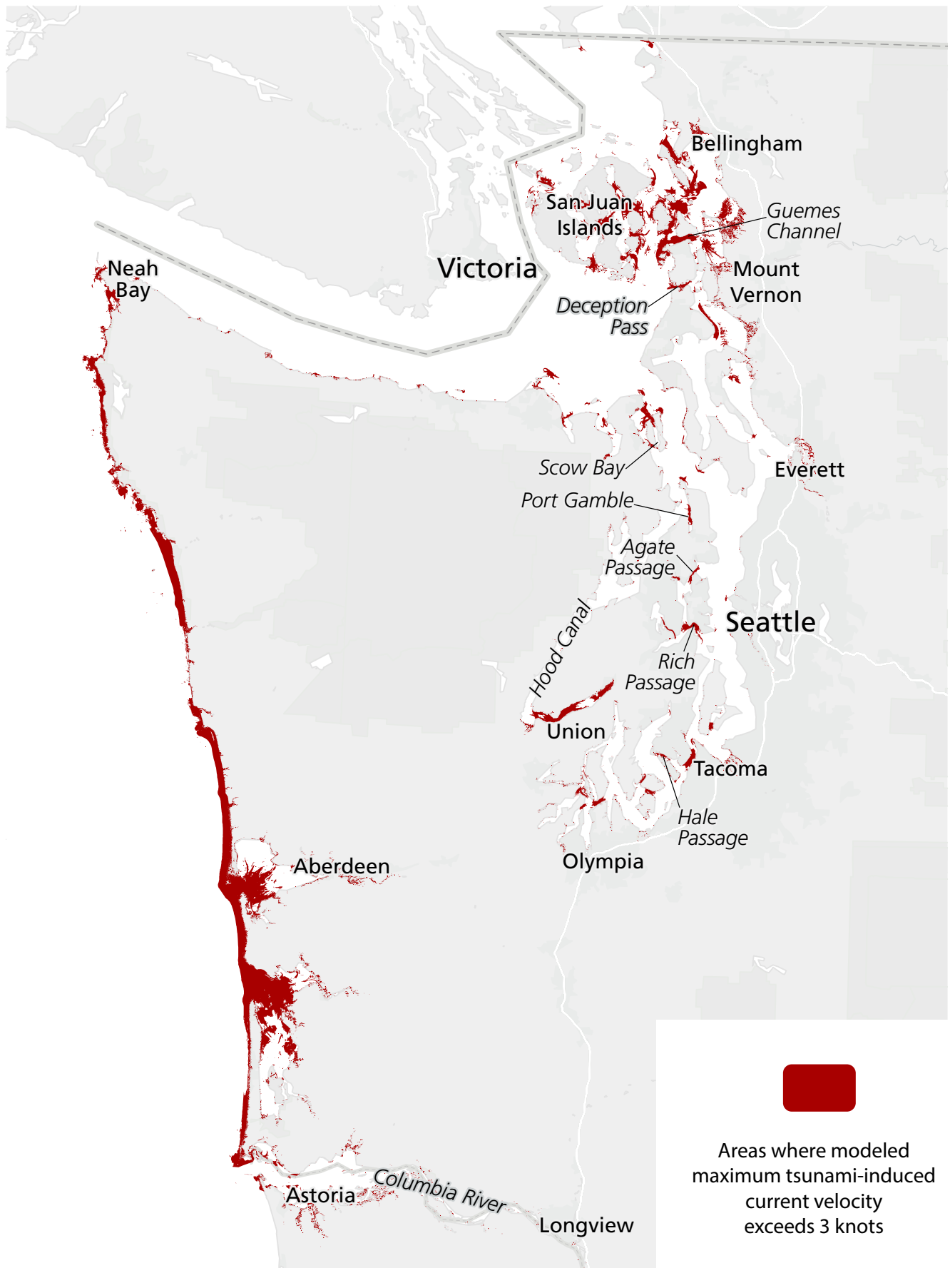
Figure 13. Map of coastal Washington showing areas where tsunami current speeds exceed 3 kn, indicating areas where damage may be expected and marine navigation would be difficult. High-speed areas may exist farther offshore along the outer coast of Washington than is depicted on this figure as we only show modeled currents up to one mile from the shoreline.
